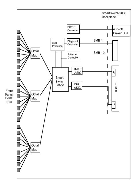
Figure 3-1. Block Diagram
